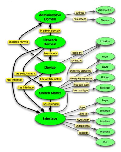
Figure 2: The main types and predicates of the NDL schema
