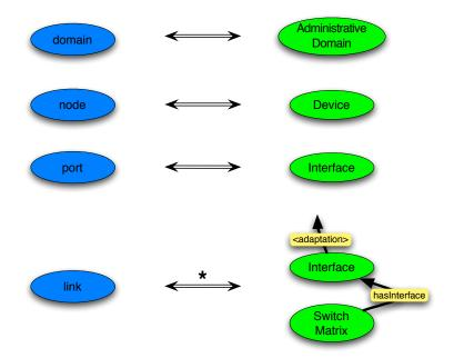
Figure 3: Mapping of objects between DCN (left) and NDL (right)
